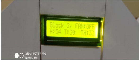
Fig 5.1: Block 2 Display showing Temperature, Humidity and fan status.
